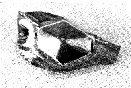
Fig. 4-6. Silicon crystal which grew in "spill-over" of a casting.
