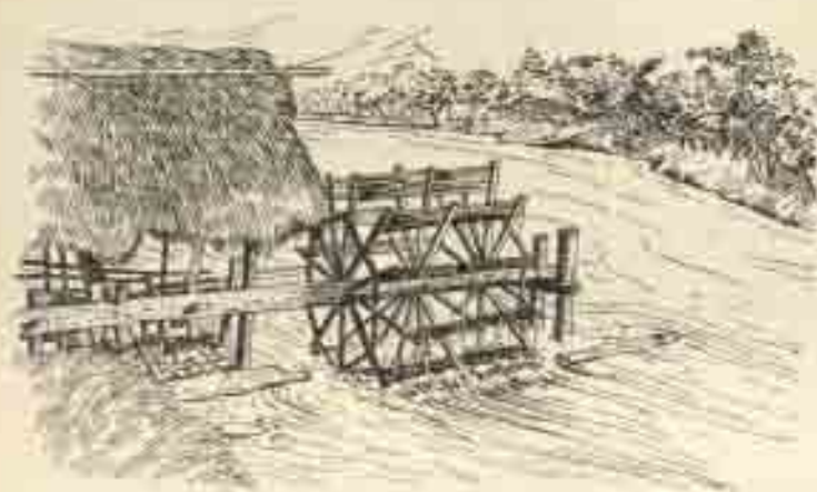
A Khumpti water-wheel which hurls paddy. Other wheels, of a different pattern, housed in small stone buildings, for grinding grain or turning prayer-wheels, are made by the Monpas and Sherdukpens of Kameng and the Membar of the Meclnka Valley.
